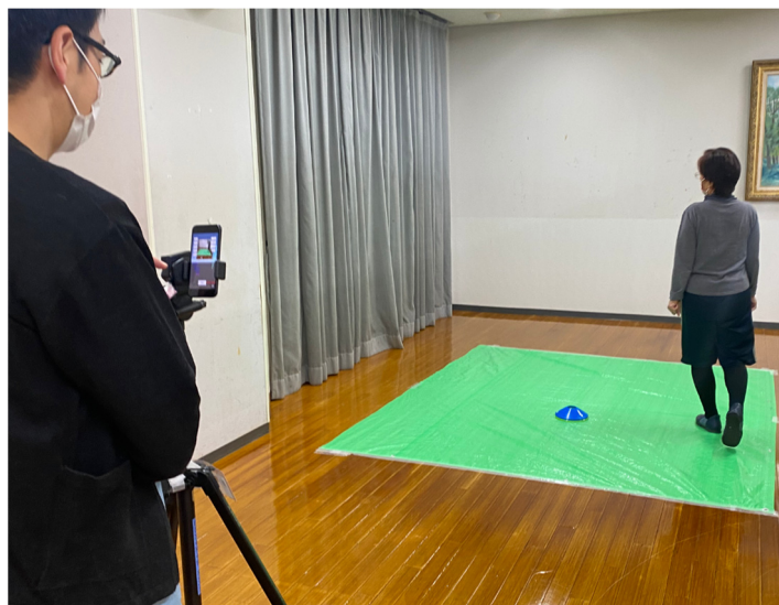
Figure 1. The markerless motion capture was recorded while the participants walked in a circle about 1 m in diameter and about 3 m away from the gait trail so that their whole body fit within the frame.
